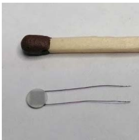
Fig. 3. Thermoelectric heat flux sensor of diameter 3 mm and height 0.7 mm.
