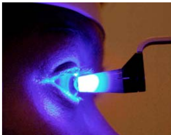
Fig. 7. Position of the contact prism fixed in Goldmann tonometer stand in the process of research with the help of a thermoelectric heat flux sensor.
