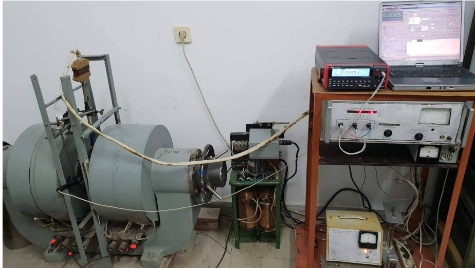
Fig. 5. General view of the device for automated measurements of thermoelectric parameters of semiconductors.
