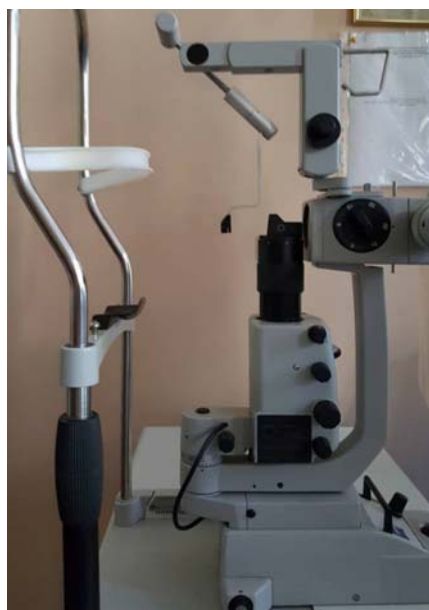
Fig. 5. Goldmann tonometer stand fixed on a biomicroscope.
