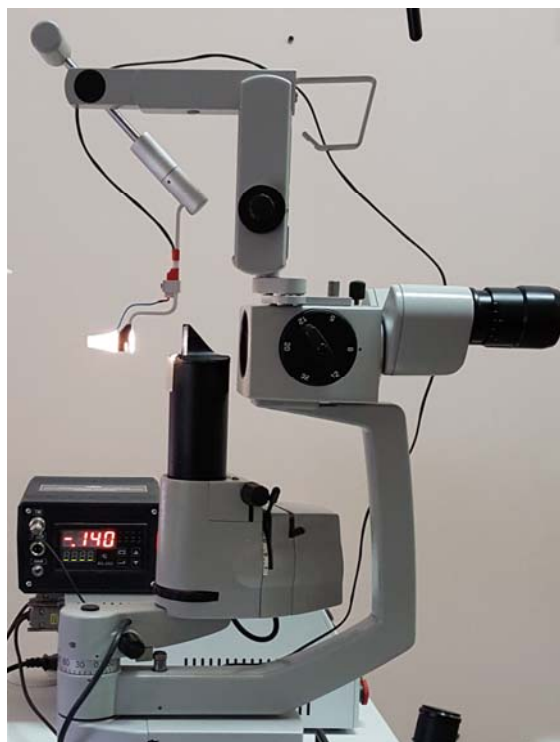
Fig. 1. Thermoelectric device for determining heat flux from the surface of the eyes: 1 – thermoelectric heat flux sensor, 2 – thermoelectric thermocouple temperature sensor, 3 – electronic control unit.
