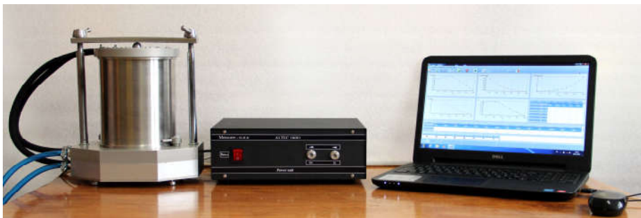
Fig. 17. External view of automated system for the determination of thermoelectric material properties in the temperature range 30 to 900 °C
