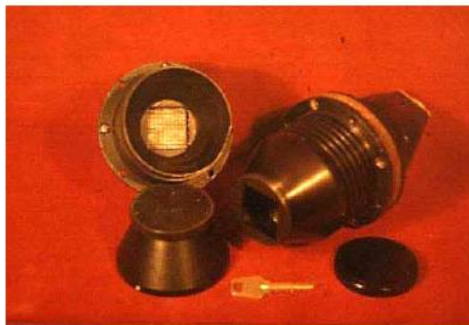
Fig.2. Matrix radiation energy receiver developed by Institute of Thermoelectricity, NAS of Ukraine
