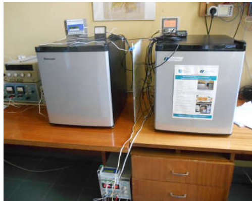
Fig. 4. Compared objects during parallel tests: on the left – the Ravanson LK-48 refrigerator, on the right - the XTT-48-1refrigerator
