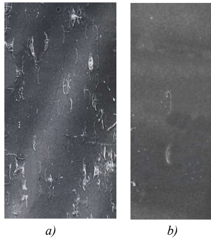
Fig. 3. Topograms of thin plate samples of CdSb. Reflection (004), a- sample edge, b – sample centre. x12.
