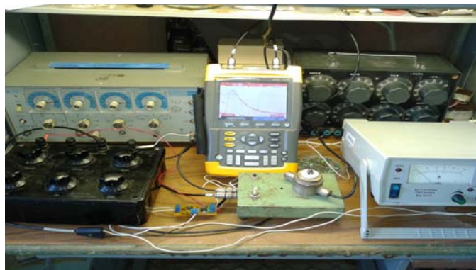
Fig. 2. The picture of a bench for measuring parameters of pulsed thermoelectric converters
