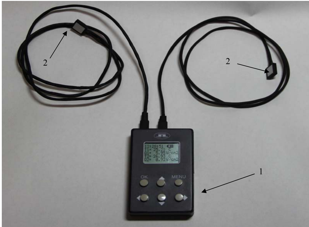
Fig. 1. Thermoelectric device for measuring temperature and heat flows: 1 – control unit, 2 – thermoelectric sensor of temperature and heat flows
