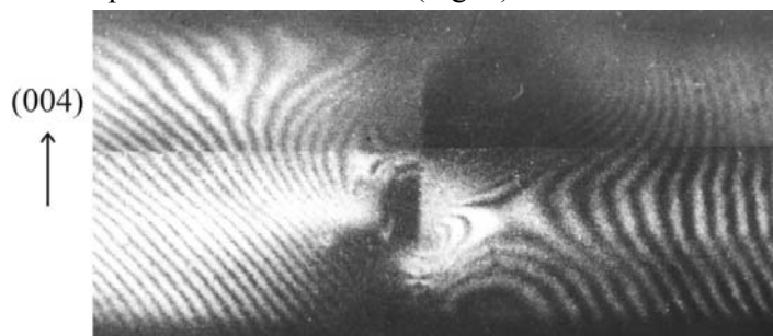
Fig. 7. Interferogram of scratches, reflection (004), \times 10 .
