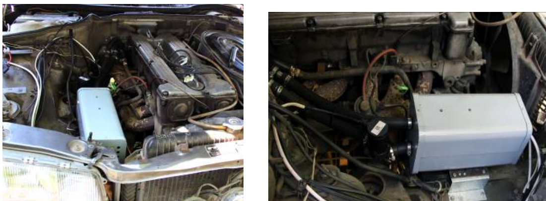
Fig. 8. Thermoelectric starting preheater in the “Mercedes” automobile.
