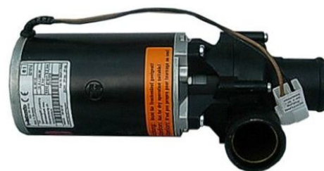
Fig. 2. Appearance of circulating pump of liquid starting pre-heater “LGW 300” (Webasto) [9].
