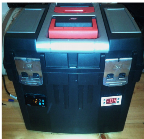
Fig. 2. Appearance of thermoelectric device prototype for storage and transportation of biological material.
