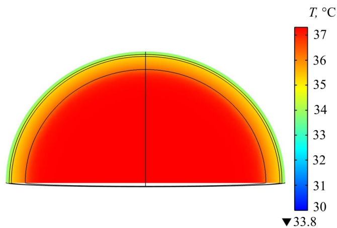
Fig. 4. The pattern of temperature distribution in the section of human head at convective heat exchange with the air at temperature + 20 °C.
