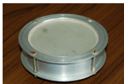
Fig. 2. Appearance of a system for cooling radio electronic equipment elements working in the intermittent heat release mode.
