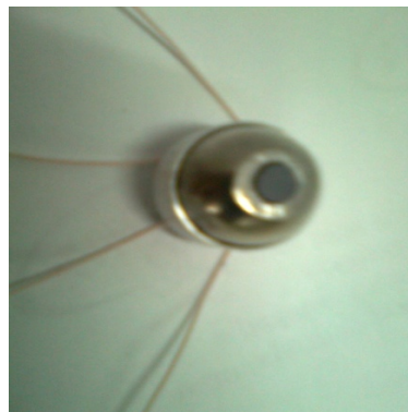
Fig. 2. External view of a detector based on anisotropic thermoelements (overall dimensions 16 × 16 mm).
