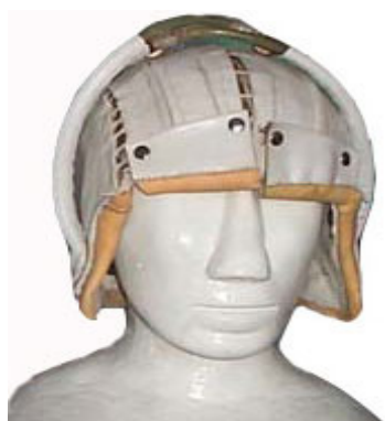
Fig.11. Helmet-shaped thermoelectric device for human head cooling (Turkey) [28]
