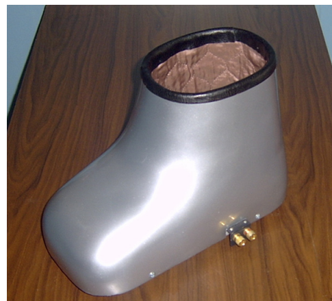
Fig. 2. Appearance of thermoelectric device for carrying out physiotherapeutic procedures.
