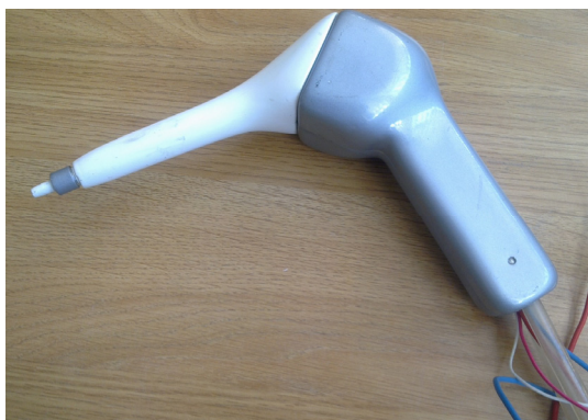
Fig. 5. External view of a system for local freezing of larynx tissues.
