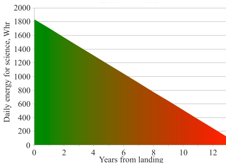
Fig. 9. Long-range energy estimate. The MSL mission uses the MMRTG to charge batteries and then draws on the batteries to conduct operations that consume high current. This plot shows how much energy should be available from the batteries as a function of time for science after accounting for the minimum energy needs of the engineering subsystems of the rover. The green section of the plot indicates there should be adequate energy to conduct all envisioned science experiments. The transition to red indicates the science experiments will likely be more limited in that timeframe.
