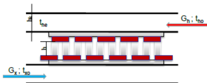
Fig.3. Design model of TEG.
