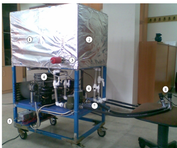
Fig. 3. The hot-cold water circulatory system. 1 – cold water storage tank, 2 – hot water storage tank, 3 – electric heater, 4 – refrigerator motors, 5 – on-off controllers, 6 – hot/cold valves, 7 – circulation motors, 8 – flowmeters.
