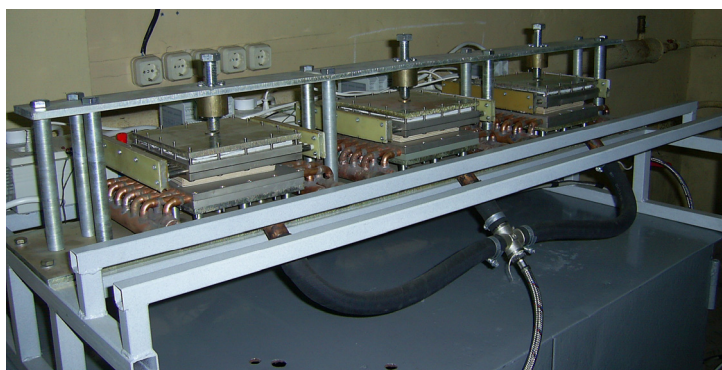
Fig. 2. Picture of installation for life test of plane-type generator thermopile.
